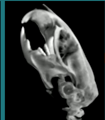
Mouse head CT, Volume rendering 45kV, 177 \mu\text{A} , 3mins scan
