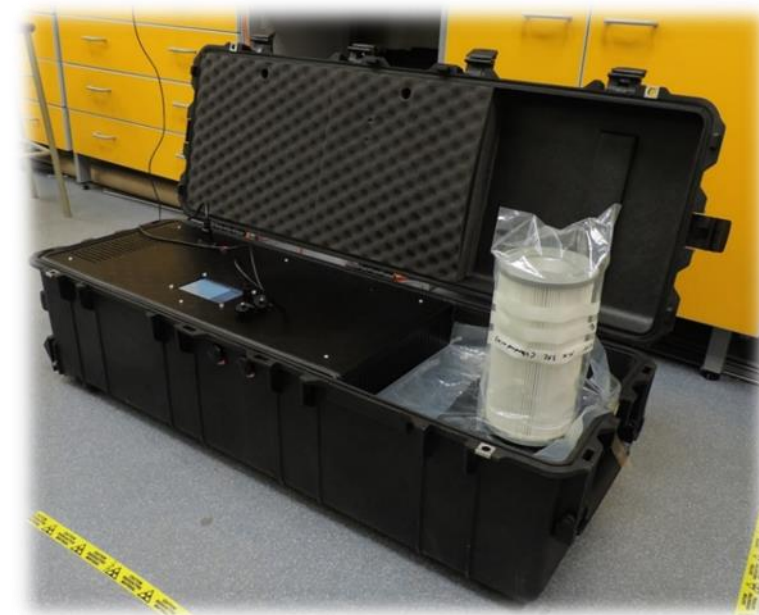
On-line aerosol particulate spectrometer ( \text{CeBr}_3 ) with high volume aerosol pump was developed and designed
