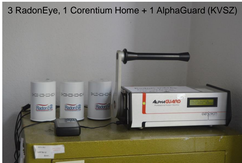
intercomparison of 5 RadonEye radon activity concentration monitors with verified AlphaGuard
